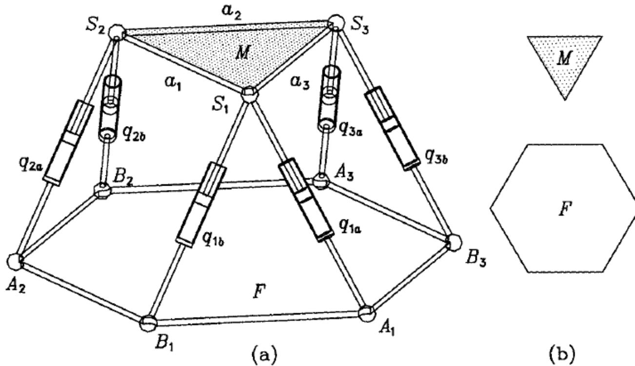
Six-dof flight simulator: (a) general layout; (b) geometry of its two platforms
