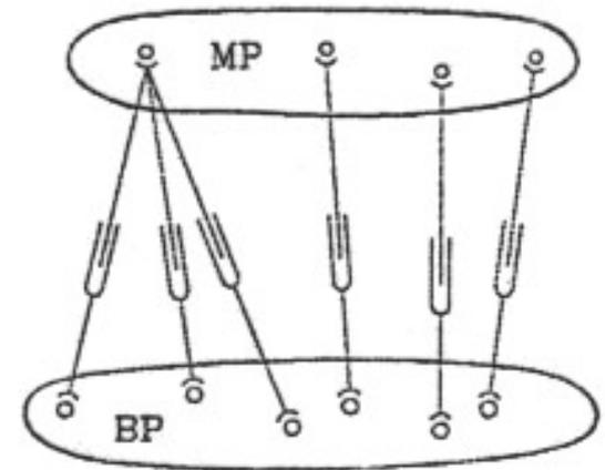
(c) A class of 6-4 structure with a triple spherical joint
