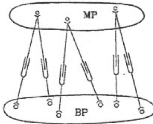
(b) A class of 6-3 structure with double spherical joints
