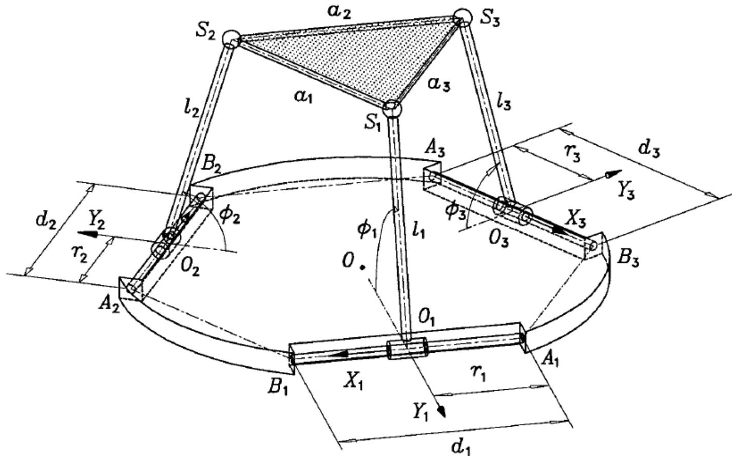
Equivalent simplified mechanism
