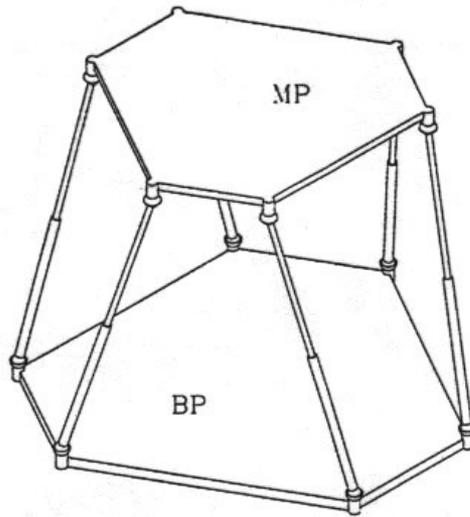
Figure 1: The six-DOF parallel manipulator with prismatic legs
