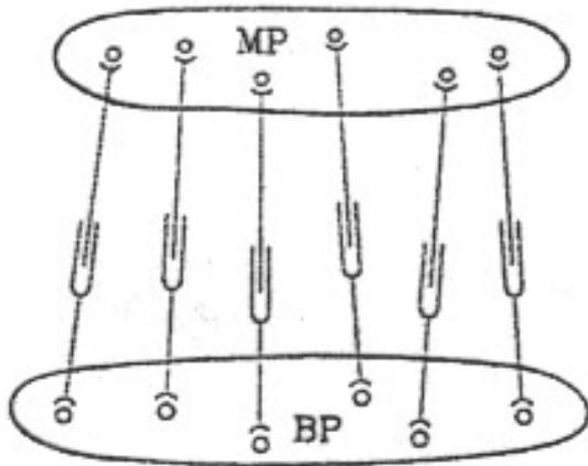
(a) The generalized 6-6 structure with single spherical joints
